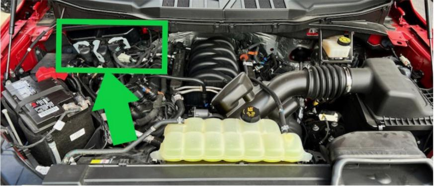
4. Be sure to release the locking tab (green arrow below) before moving gray connector arm. Disconnect all 3 of the ECU connectors.
