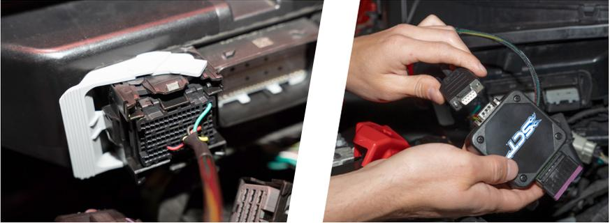
6. Connect the X4 to the SCT box using the OBDII cable,
